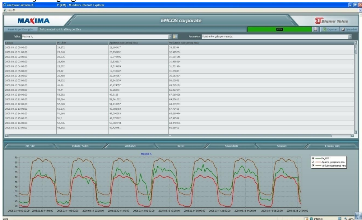
Consumption of electric power (the green line) deviates from the average consumption schedule by more than the dynamic limit set by the user for three nights in succession (detected by the system automatically)
